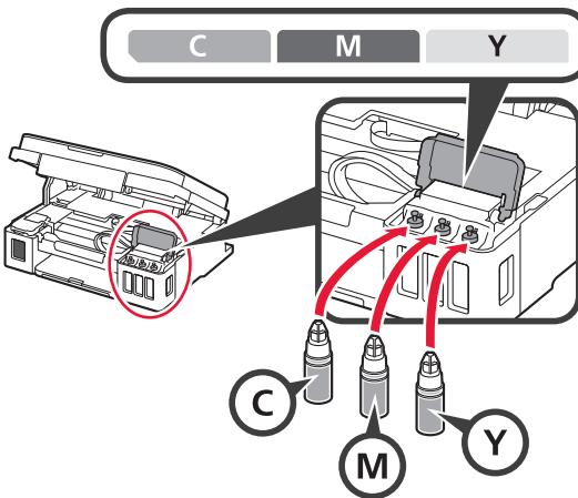
Confirm that the ink has been filled to the upper limit line (A).
