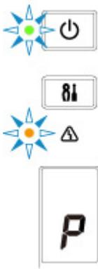
The error code appears on the LCD one by one.
