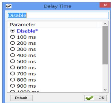
Sets the Delay Time between every tag scan. This feature may be disabled by setting Delay Time to 0 (Disabled).
