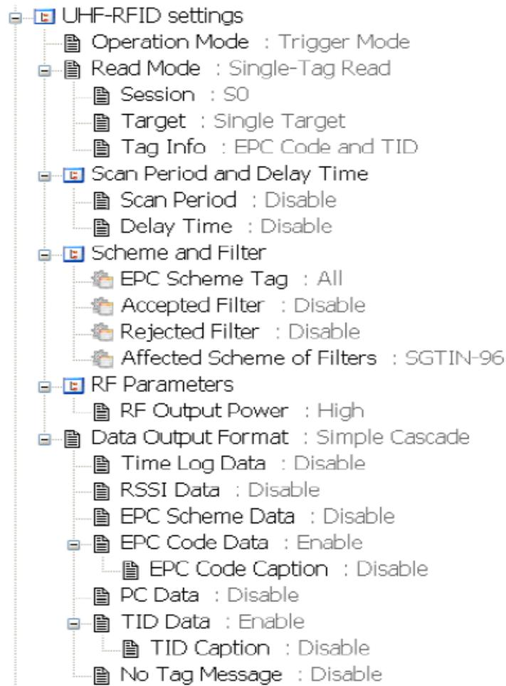
Choose the item to configure, then double click the left mouse button or press Enter to enter the desired parameters setting window.
