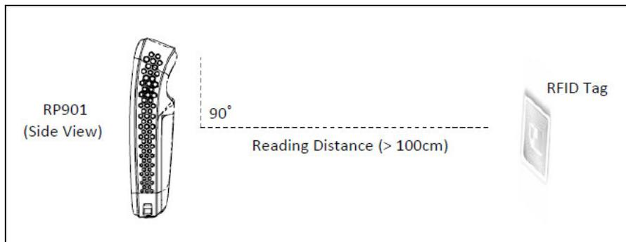
**CAUTION!** Reading distance may be impacted by the type of tag and environmental conditions. The graphic above is based on Alien 964X Higgs-3 tag and tested in an office environment (25°C)
