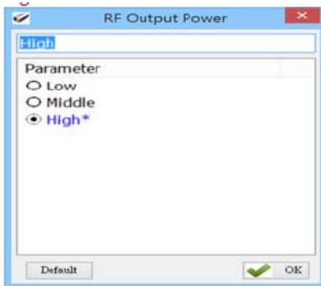
Configuration Method: Select one RF output power level then click  OK to send the new parameter value to the RP901.
