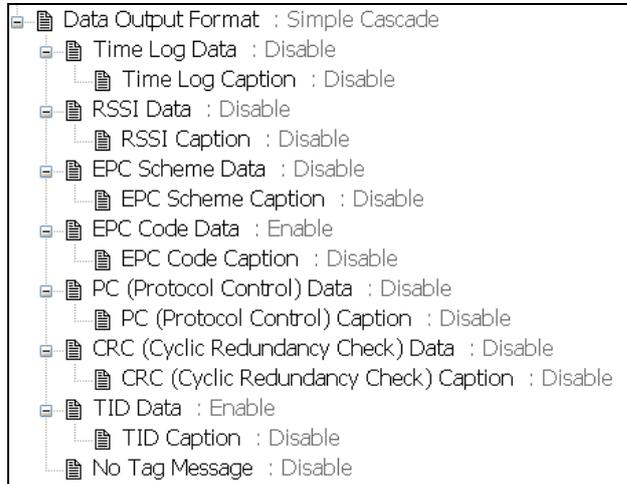
The Data Output Format options include settings for Time Log, RSSI, EPC Scheme, EPC Code, PC (Protocol Control), CRC (Cyclic Redundancy Check) and TID data.
