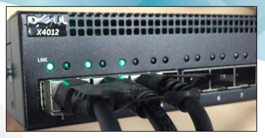
You can connect the power to the switch now, which will automatically power on. The default configuration for the X4012 is an isolated (default) single VLAN. The switch will not require any configuration as the goal is to have an isolated, non-routed network for node-to-node backplane communication only.
